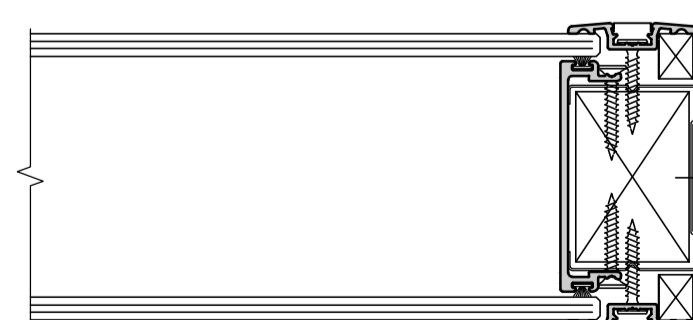
SECTION O DOUBLE GLAZED / STRUCTURE (TRIMMED ABUTMENT)
